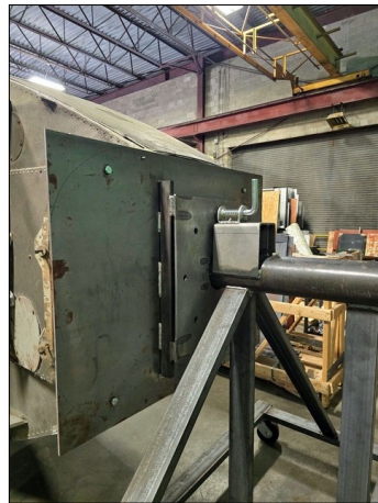
Above: Rotisserie front and rear panel connections
