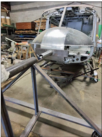
Above: Rotisserie front and rear panel connections
