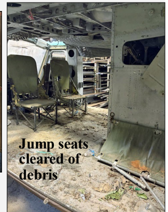
Top of photo is the ceiling of the Huey; jump seats were packed with fuel bladders and extra parts
